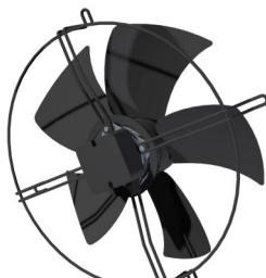
Helical fan with profiled blades to increase efficiency and minimize sound level, directly coupled to the electric motor, mono-phase with external rotor, VDE compliant, with built-in thermal protection. It is housed in aerodynamically shaped flow nozzles.
